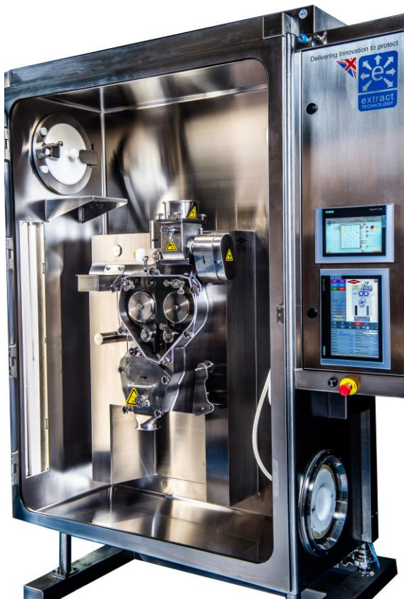
Fitzpatrick CCS 320 integrated into Extract Technology containment isolator
