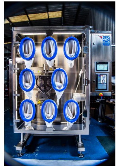
Completed isolator providing OEB 5 containment with integrated compactor
