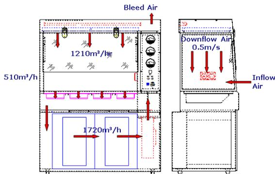
Airflow is introduced through the open sash aperture to ensure contaminants are contained within the work area. The bench itself is provided on castors with a flying lead and plug for connection to a power supply.
