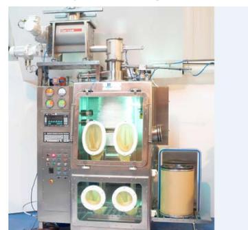
The entire process ensures operator safety from potent APIs (active pharmaceutical ingredients) while minimising cross contamination risks.
