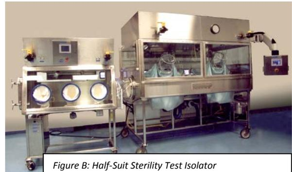
Figure B: Half-Suit Sterility Test Isolator
