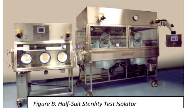
Figure B: Half-Suit Sterility Test Isolator
