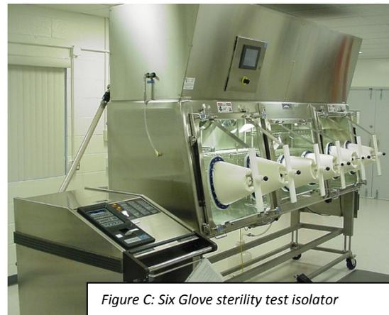
Figure C: Six Glove sterility test isolator
