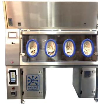
Figure A: Simple sterility test isolator
