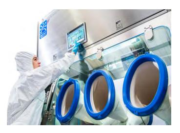
The solution consisted of an isolator with a transfer airlock, main chamber with integrated weighing system and a rapid transfer port to achieve OEL of <1µg/m³. Furthermore a GEA high containment split butterfly valve was integrated into the base of the machine for safe transfer of API to the mobile vessel docked below. A static platform was included to raise the isolator allowing a mobile vessel to dock with a high containment split butterfly valve on the outlet of the isolator.
