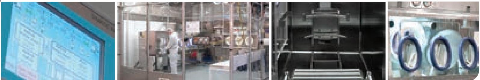
Extract Technology Rigid Containment Isolators have been designed for handling potent compounds that can offer guaranteed levels of operator protection as low as 10ng/m<sup>3</sup> (task duration). These include designs for sampling, dispensing and sub-division, mixing, milling and vessel charging, as well as containing integrated process devices such as filter dryer units, tablet press enclosures, blenders, mills and pack off systems.
